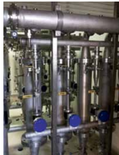
Degassed Pig Manure, Denmark: LiqTech's SiC membranes used for UF stage. Capacity: 12 m 3 /h.
