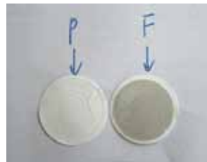
From the SDI measurement: Permeate (left), feed (right)
