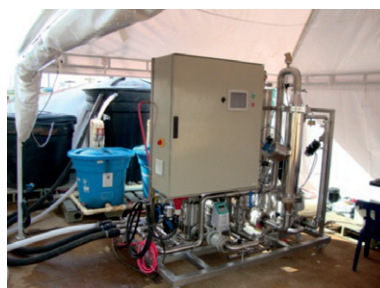
Case 2 - Test setup with automatic pre-filtration (300 µm), CIP unit and LiqTech's MultiBrain membrane filtration unit
