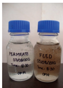
Case 2 - Samples from the field trials: Permeate (left) and feed (right)
